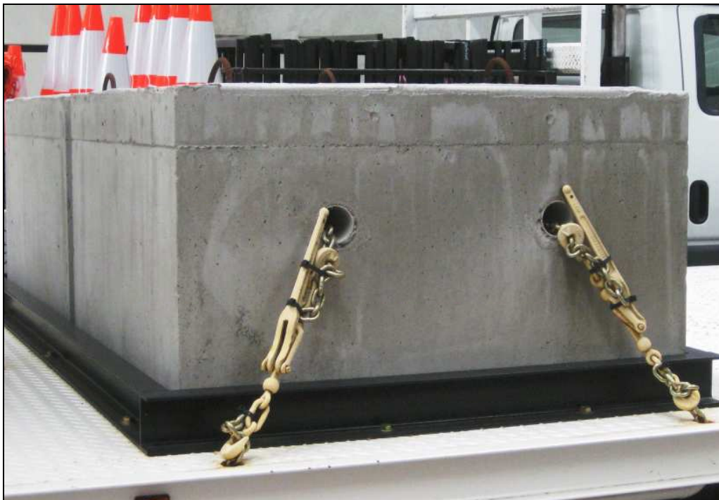
A frame to prevent sliding and chain type tie downs observed during a recent site visit as an example of a ballast restraint device currently in use.
