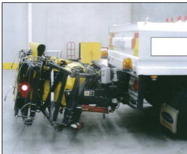
The crash attenuator was fully compressed by the high speed impact
